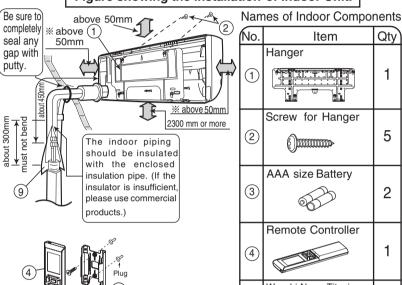
**Direction of Piping** Backward piping from left Connection There are 6 directions allowed,namely,backward
